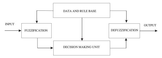
Figure 1. General structure of a fuzzy control system.
