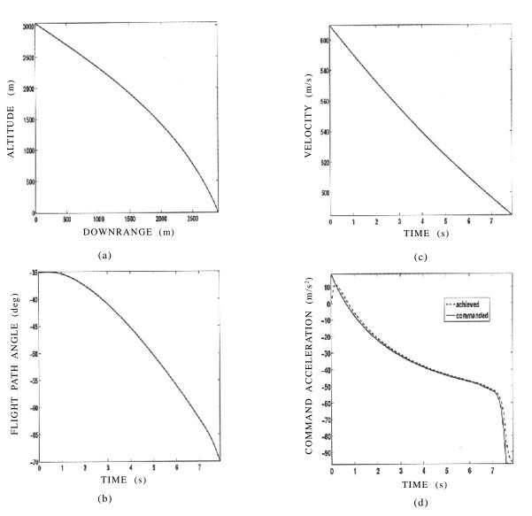
Figure 4. Performance of fuzzy logic guidance: (a) Missile trajectory, (b) missile flight-path angle history, (c) missile velocity history, and (d) commanded acceleration history.
