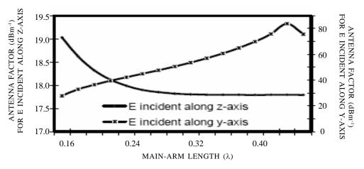
Figure 12. Antenna factor (dBm<sup>-1</sup>) versus length in wavelengths of I-shaped antenna.
