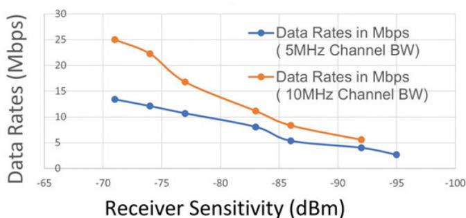
Figure 9. Receiver sensitivity and data rates.
