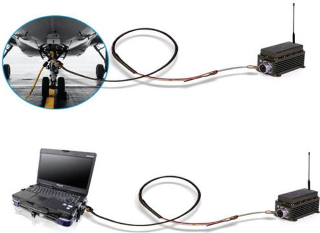
Figure 2. Overall setup of the aircraft to ground wireless transfer.
