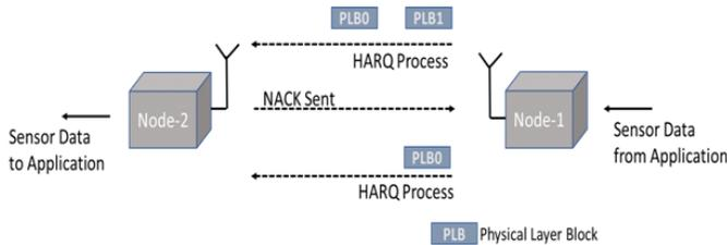
**Figure 10. Physical layer block level re-transmission.**
