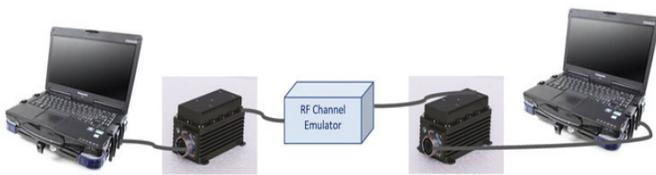
Figure 8. Lab-based controlled conduction test setup.
