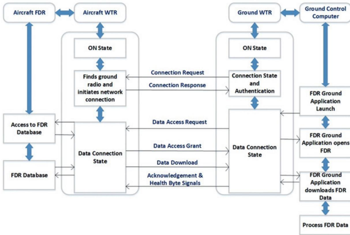
Figure 6. Data transfer state machine.
