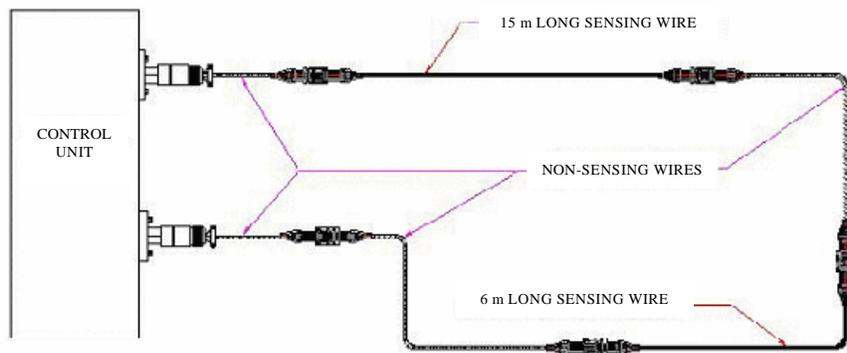
**Figure 1. Requirement of 15 m and 6 m long sensing wires without any joint.**
