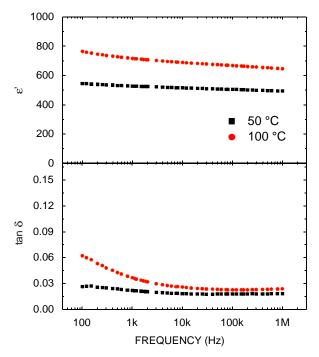
Figure 6. Frequency dependence of  $\varepsilon$ ' and tan  $\delta$  at different frequencies for x = 0.02.
