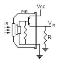
Figure 2. Single-element pyroelectric detector.
