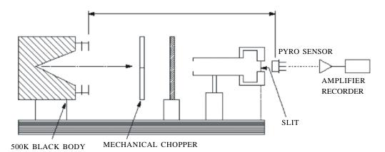
Figure 8. Experimental setup for detectivity and responsivity measurement of the pyro sensors.
