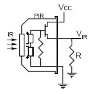
Figure 3. Dual-element pyroelectric detector.
