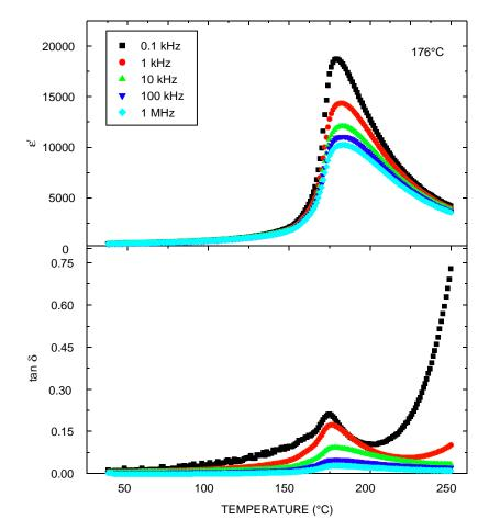
Figure 5. Temperature dependence of  $\varepsilon'$  and tan  $\delta$  at different frequencies for x = 0.02.
