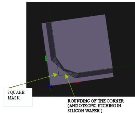
Figure 2. Simulation with AnisE module.
