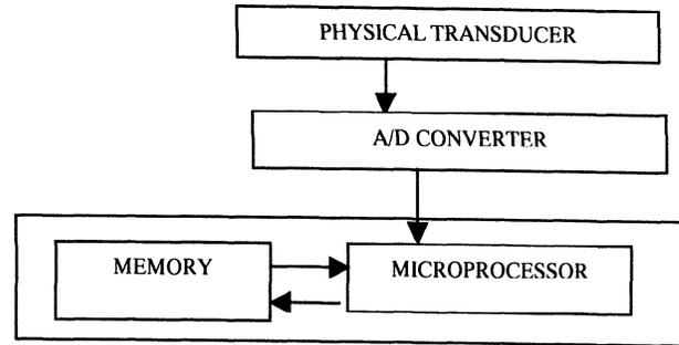
Figure 1. Smart sensor model.
