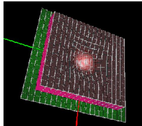
Figure 3. Simulation of membrane under pressure with MEMS design software.
