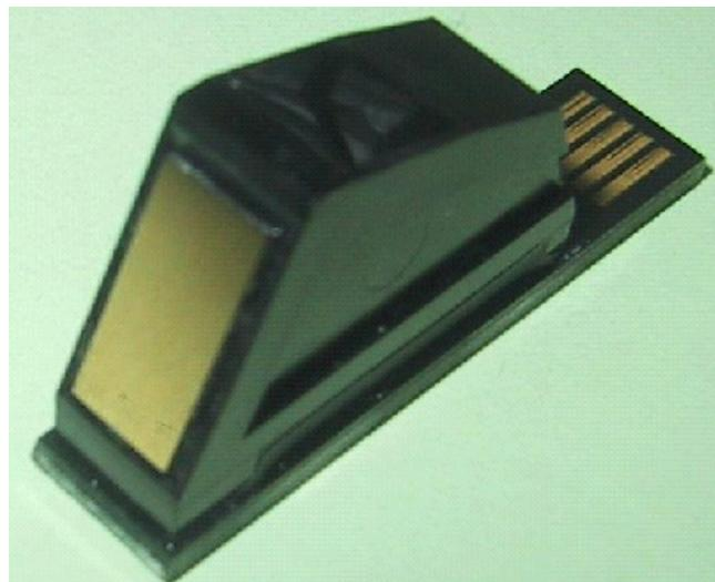
**Figure 2. Integrated surface plasmon resonance sensor Spreeta 2000 suitable for design of portable SPR biosensors.**
