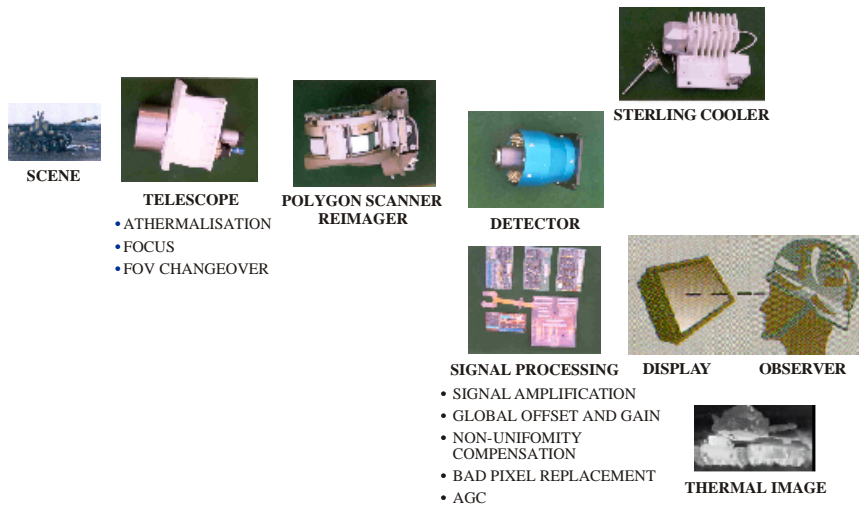
Figure 4. Subsystems of a thermal imaging system.
