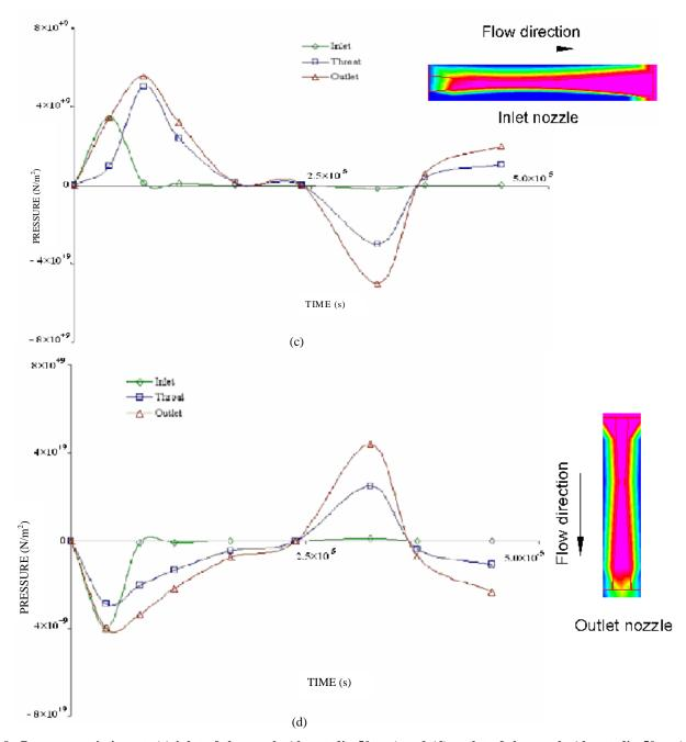
Figure 9. Pressure variation at: (c) inlet of the nozzle (throat dia 50 µm) and (d) outlet of the nozzle (throat dia 50 µm).
