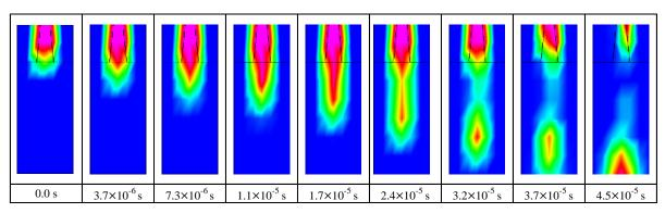
Figure 4. Tailing effect and droplet formation for fully wetting substrate (nozzle dia 38 µm and 5.0 vol % of alumina in ethanol).
