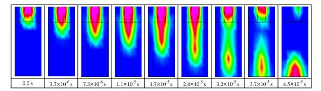
Figure 7. Tailing effect and droplet formation for fully wetting substrate (nozzle dia 50 µm and 7.5 vol % of alumina in ethanol).
