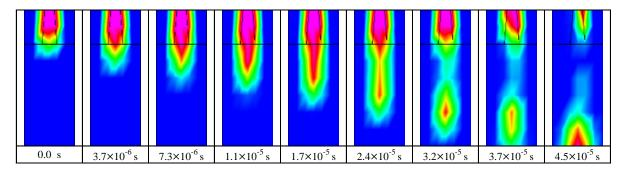
Figure 5. Tailing effect and droplet formation for fully wetting substrate (nozzle dia 38 µm and 7.5 vol % of alumina in ethanol).
