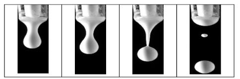
Figure 3. Tailing while droplet formation and ejection.
