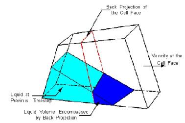
Figure 2. Back projection concept for the PLIC scheme.
