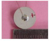
Figure 15. Piezoelectric actuator with electrodes fixed.
