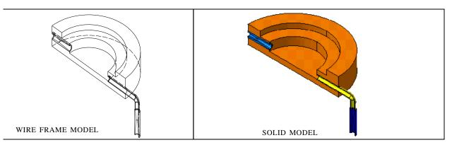
Figure 13. Chamber and nozzle assembly in CAD.
