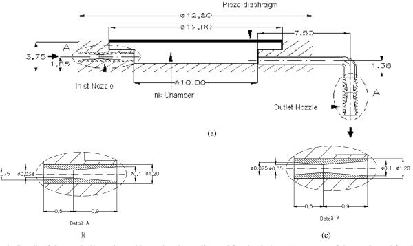
Figure 1. Details of the nozzle dimensions with varying throat dia. used for simulation: (a) geometry of the nozzle used for simulation of droplets, (b) nozzle with 0.038 mm throat dia, and (c) nozzle with 0.05 mm throat dia. (all dimensions in mm)
