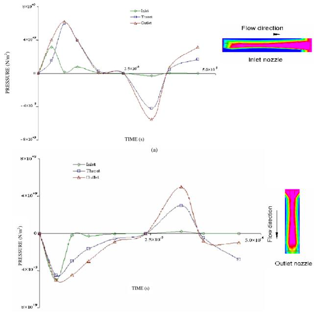
Figure 8. Pressure variation at: (a) inlet of the nozzle (throat dia 38 µm), (b) outlet of the nozzle (throat dia 38 µm).
