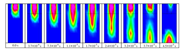
Figure 6. Tailing effect and droplet formation for fully wetting substrate (nozzle dia 50 µm and 5.0 vol % of alumina in ethanol).
