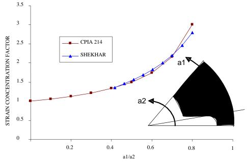
Figure 8. Comparison of strain concentration factors.
