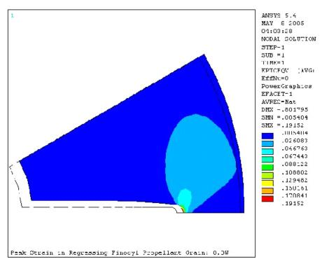
Figure 2. Equivalent strain in initial finocyl port configuration.
