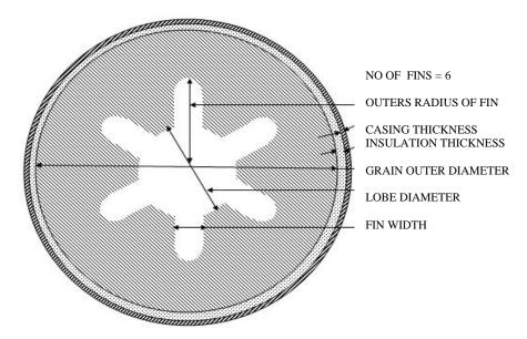
Figure 1. Geometrical parameters of finocyl port case bonded propellant.
