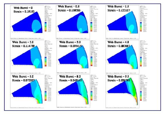
Figure 3. Peak strain variation in 6 fin initial finocyl.
