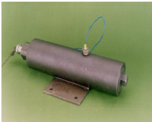
Figure 1. Photograph of atypical closed vessel.
