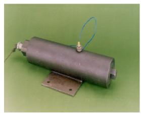
Figure 1. Photograph of atypical closed vessel.
