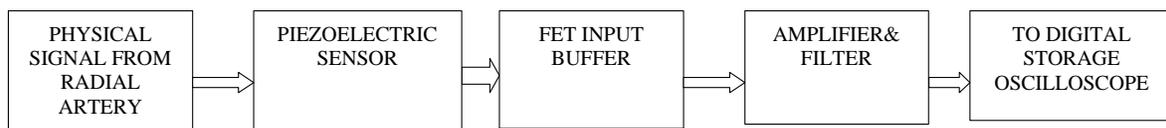
Figure 2. Block diagram of pulse detection system using digital storage oscilloscope.
