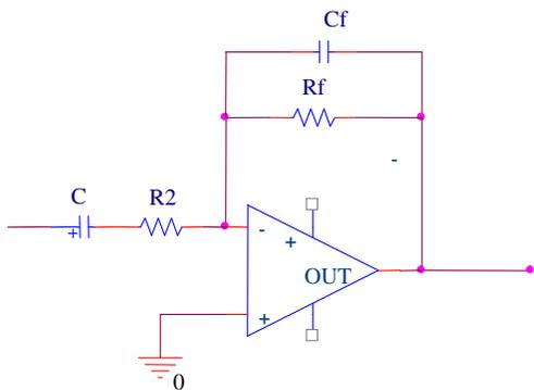
Figure 4. Low-pass filter/amplifier.
