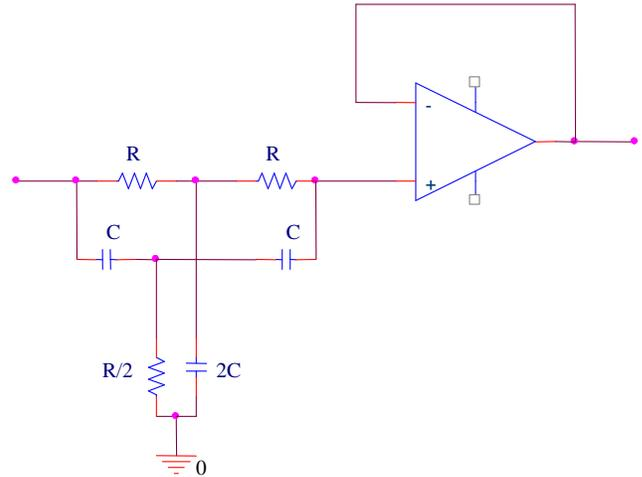
Figure 5. Notch filter.
