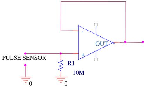
Figure 3. FET input buffer amplifier.
