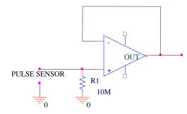
Figure 3. FET input buffer amplifier.
