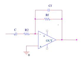
Figure 4. Low-pass filter/amplifier.
