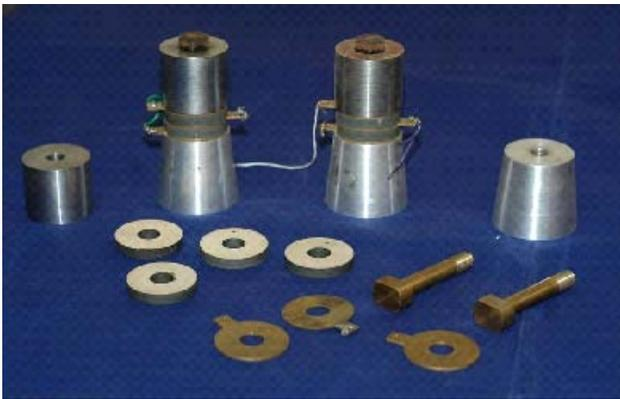
Figure 2. Components used in piezoceramic-based transducer system.
