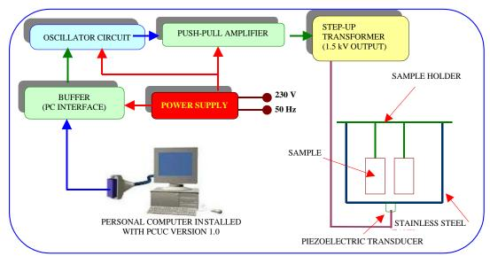
Figure 3. Schematic diagram of PC-based ultrasonic cleaner.
