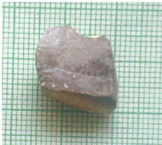
Figure 2. Grown PZN-PT (91-9) single crystal by bottom-supported flux Bridgman method.
