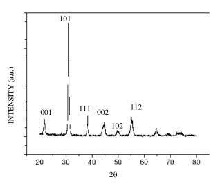
Figure 2. XRD pattern of calcined PNN-PZT.
