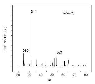
Figure 1. XRD pattern of calcined NN (NiNb,O<sub>6</sub>).
