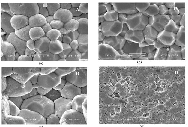
Figure 4. SEM of polished and chemically etched surfaces of the specimens sintered at 1280 °C for 4 h: Heating rate (a) 14 °C/min, (b) 8 °C/min, (c) 6 °C/min, and (d) 3.5 °C/min.
