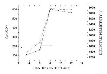
Figure 3. Variation of dielectric constant and piezoelectric charge constant with heating rate.
