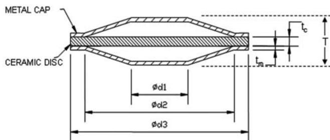
Figure 1. Schematic of the cymbal transducer.
