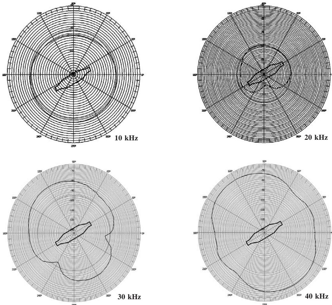
Figure 4. Receiving directivity of PNS-PZT hydrophone.
