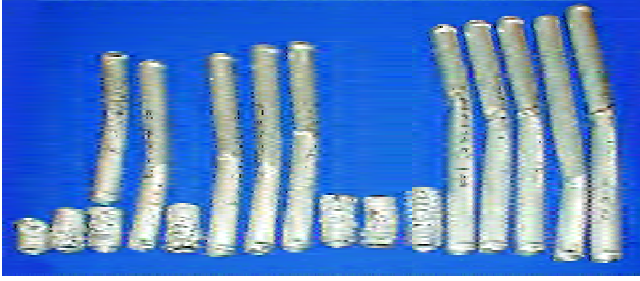
Figure 3. Final deformation profiles of aluminium alloy 6063-T6 circular tubes with increasing initial length from left to right and crushed quasi-statically at 2 mm/min 24 .
