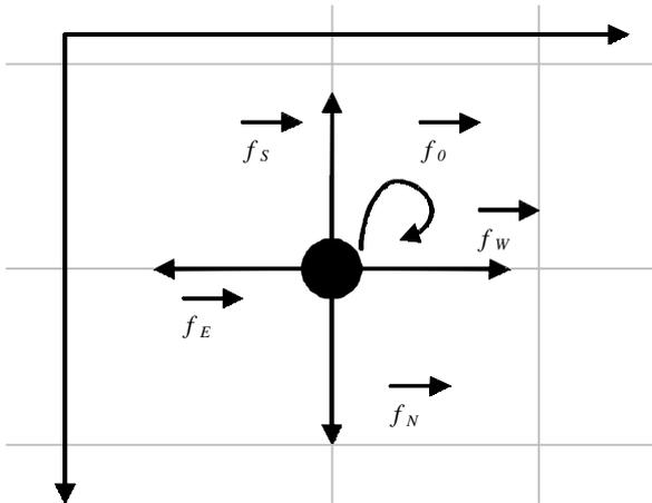
Figure 3. ParFlow node and its outward flow.
