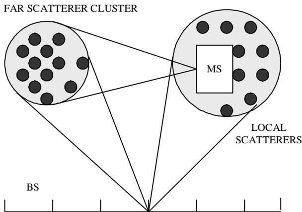
Figure 4. Geometry-based stochastic channel model.
