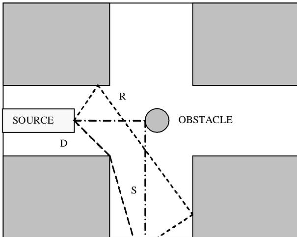
**Figure 1. Basic propagation mechanisms – reflection (R), diffraction (D), and scattering (S).**
