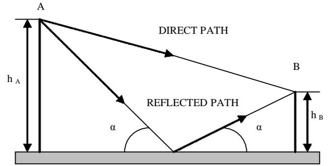
Figure 6. Geometrical two-ray model.
