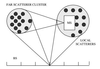
Figure 4. Geometry-based stochastic channel model.
