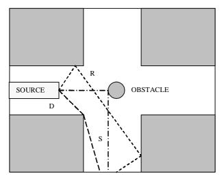
Figure 1. Basic propagation mechanisms – reflection (R), diffraction (D), and scattering (S).
