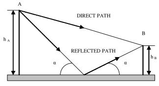
Figure 6. Geometrical two-ray model.
