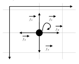
Figure 3. ParFlow node and its outward flow.
