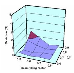
Figure 2. Percentage deviation in the computed values of plasma frequency reduction factor using Eqn (4) wrt (Table 1).
