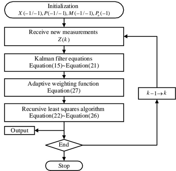
Figure 3. Flowchart of the adaptive input estimation algorithm.
