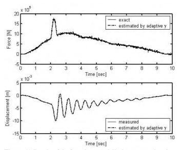
Figure 11. Results of the force input and displacement estimation under the multiple tank and single missile impact force inputs.  $(F_1 = F_2 = F_3 = 500 \text{ (KN)}, v_1 = 8, v_2 = 6, v_3 = 4 \text{ m/s}, Q_W = 10^9, R_V = 10^{-12}, \text{ and error} = 5.13 \text{ per cent)}.$
