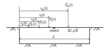
Figure 2. The bridge structure model under the moving multiple tank and missile impact force inputs.
