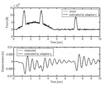
Figure 8. Results of the force input and displacement estimation under the singular tank and triple missile impact force inputs.  $(Q_w = 10^9, R_v = 10^{-12}, x_1 = L/2, x_2 = L/3, x_3 = 2L/3,$ and error= 10.45 per cent).
