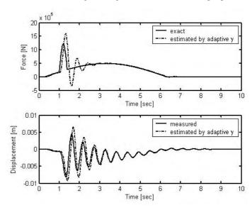
Figure 5. Results of the force input and displacement estimation under the singular tank and single missile impact force inputs. ( $Q_w = 10^4$ ,  $R_v = 10^{-12}$ ,  $x_1 = L/2$ , and error= 48.83 per cent).
