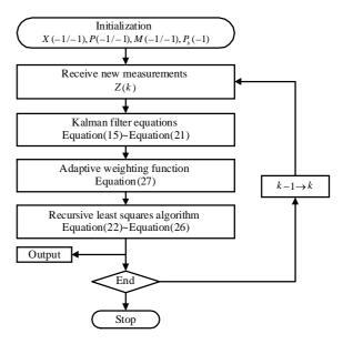
Figure 3. Flowchart of the adaptive input estimation algorithm.
