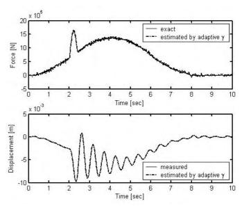
Figure 10. Results of the force input and displacement estimation under the multiple tank and single missile impact force inputs.  $(F_1 = F_2 = F_3 = 500(\text{KN}), v_1 = v_2 = v_3 = 5 \text{ m/s}, Q_W = 10^9, R_V = 10^{-12}, \text{ and error} = 4.29 \text{ per cent}).$
