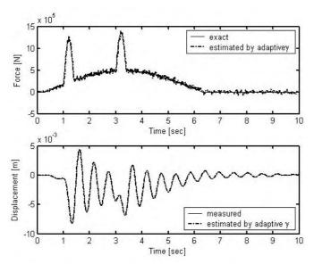
Figure 7. Results of the force input and displacement estimation under the singular tank and double missile impact force inputs.  $(Q_w = 10^\circ, R_v = 10^{-12}, x_1 = L/2, x_2 = L/3 \text{ and error} = 9.80 \text{ per cent}).$
