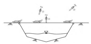
Figure 1. Bridge structure system under moving tank and missile impact loads.
