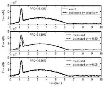
Figure 9. Comparison of the inverse estimation using the fuzzy, and constant weighting functions under the singular tank and single missile impact force inputs.  $(Q_{\rm w}=10^{\rm 9},\,R_{\rm v}=10^{\rm -10},\,x_{\rm i}\!=\!\!L/2).$
