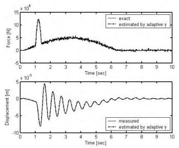
Figure 6. Results of the force input and displacement estimation under the singular tank and single missile impact force inputs.  $(Q_w = 10^9, R_v = 10^{-12}, x_1 = L/2, \text{ and error} = 10.03 \text{ per cent}).$
