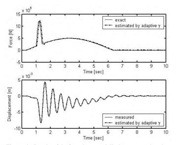
Figure 4. Results of the force input and displacement estimation under the singular tank and single missile impact force inputs.  $(Q_w = 10^4, R_v = 10^{-14}, x_1 = L/2, \text{ and error} = 20.44 \text{ per cent}).$
