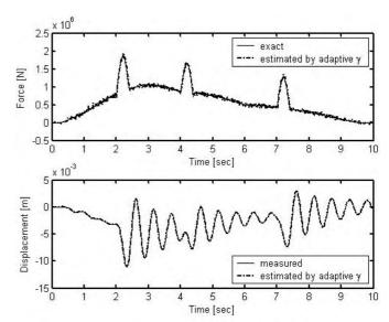
Figure 13. Results of the force input and displacement estimation under the multiple tank and triple missile impact force inputs. ( $F_1 = F_2 = F_3 = 500(\text{KN})$ ,  $v_1 = 8$ ,  $v_2 = 6$ ,  $v_3 = 4$  m/s,  $x_1 = L/2$ ,  $x_2 = L/3$ ,  $x_3 = 2L/3$ ,  $Q_W = 10^9$ ,  $R_V = 10^{-12}$ , and error = 6.00 per cent).
