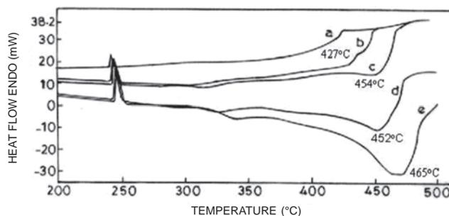
Figure 3. DSC of AP + 0.5 %  $Fe_2O_3$  (3.5 nm) at different heating rates: (a) 5 °C/min, (b) 10 °C/min, (c) 15 °C/min, (d) 20 °C/min, and (e) 25 °C/min.
