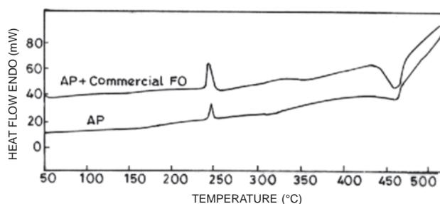
Figure 2. DSC of pure AP and AP + 2 % commercial  $Fe_2O_3$  (FO) at 10 °C/min.
