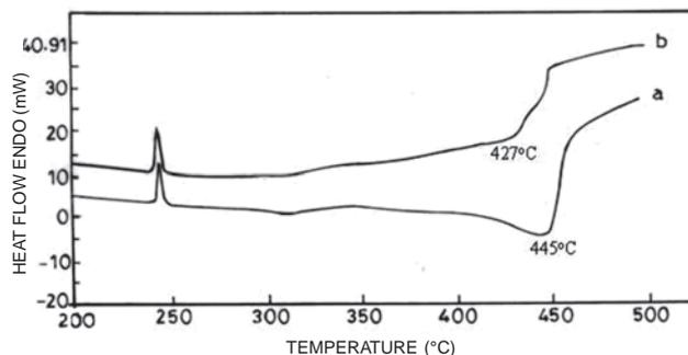
Figure 4. DSC of AP+ 0.5 Wt %  $Fe_2O_3$  at different particle sizes: (a) 30 nm and (b) 3.5 nm at 10 °C/min.
