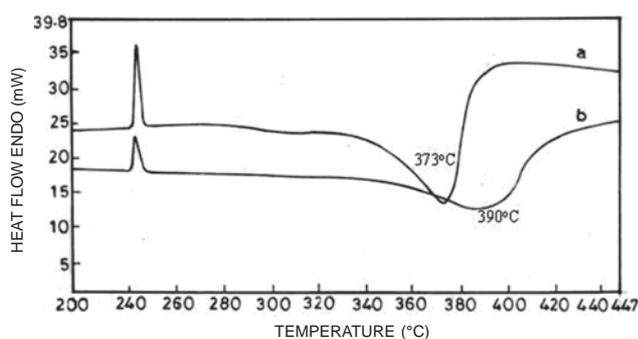
Figure 7. DSC of AP+ 5 Wt %  $Fe_2O_3$  at different particle sizes: (a) 30 nm and (b) 3.5 nm at 10 °C/min.
