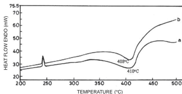
Figure 6. DSC of AP+ 2 Wt %  $Fe_2O_3$  at different particle sizes: (a) 30 nm and (b) 3.5 nm at 10 °C/min.
