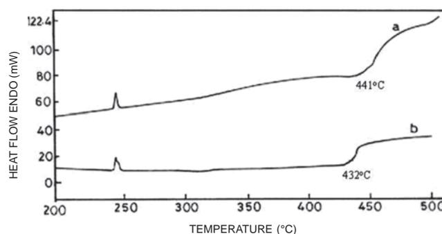
Figure 5. DSC of AP+ 1 Wt %  $Fe_2O_3$  at different particle sizes: (a) 30 nm and (b) 3.5 nm at 10 °C/min.
