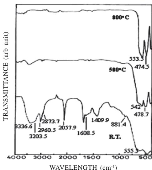
Figure 1. FTIR spectra of as prepared  $Fe_2O_3$  and after annealing at 500 °C and 800 °C.
