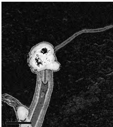
Figure 13. Typical TEM micrograph of a PECVD sample showing carbon nanotubes growing in different direction from a lump of catalyst.
