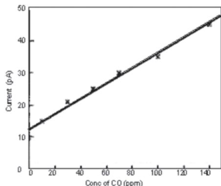
**Figure 9.** Plot of concentration of CO versus current for the sensor based on nanocomposite of aluminum doped iron oxide in a copolymer matrix of aniline-formaldehyde.
