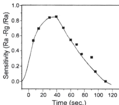
Figure 5. Response of the  $\text{SnO}_2$ : $\text{Pd}$  thick film to 200 ppm LPG at 200 °C.
