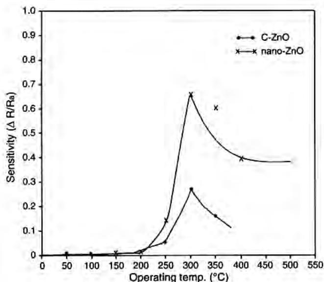
Figure 6. Sensitivity as a function of operating temperature of: (a) nano-ZnO and (b) C-ZnO exposed to 100 ppm  $NH_3$  gas at 300 °C.
