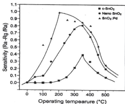
Figure 3. Temperature dependence of the sensitivity of  $\text{SnO}_2$  thick films at different operating temperatures.
