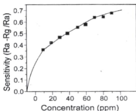
Figure 4. Sensitivity as a function of different concentrations of LPG gas at 200 °C.
