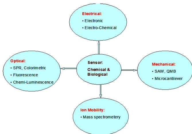
**Figure 2. Classification of sensor technologies based on their energy transduction.**
