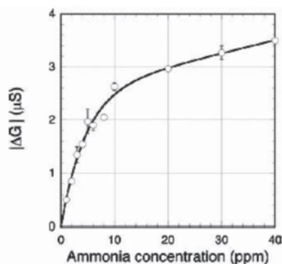
**Figure 19.** Conductance change of the MWCNTs gas sensor as a function of ammonia. (Reproduced<sup>51</sup> with permission from Institute of Physics, UK, 2003).
