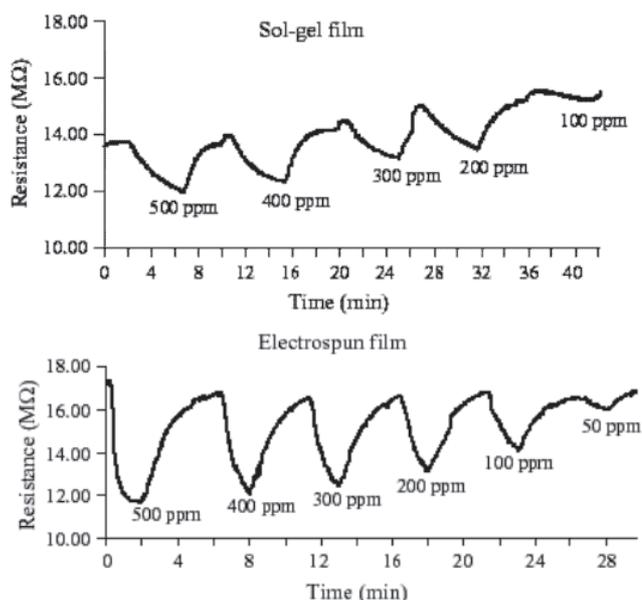
Figure 12. (a) Sensing data for the sol-gel-based  $WO_3$  thin film's response to  $NO_2$  and (b) Sensing data for the nano-fibre-based  $WO_3$  film response to  $NO_2$ . (Reproduced<sup>35</sup> with permission from Elsevier Science, 2005).
