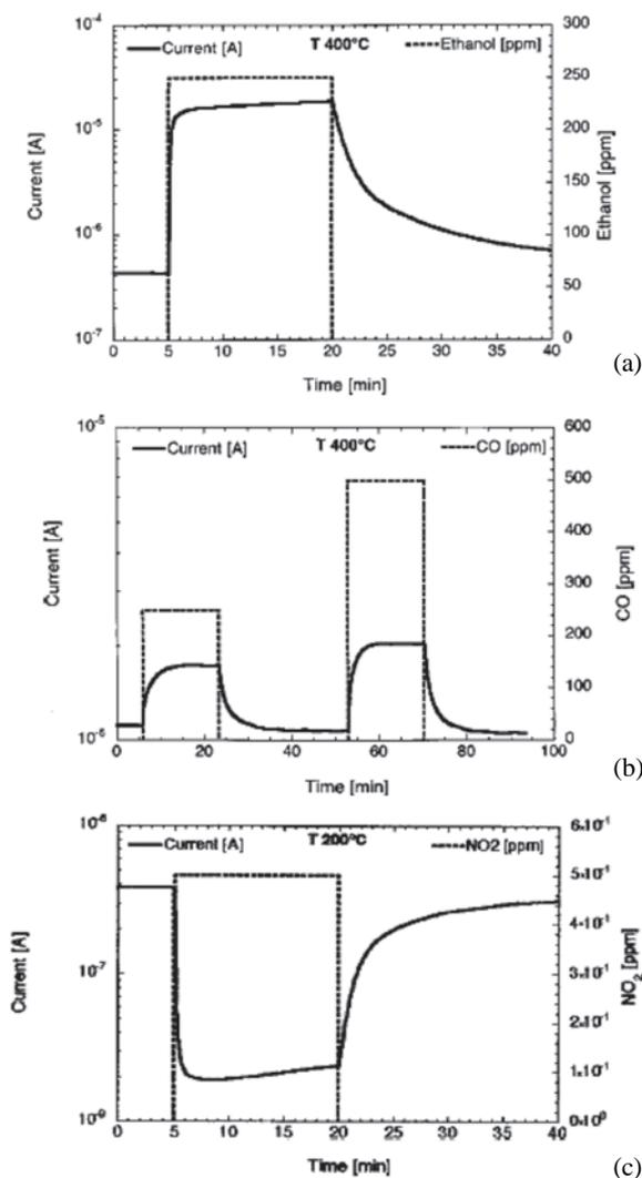
Figure 20. (a) Response of the  $\text{SnO}_2$  nanobelts to ethanol at a working temperature of  $400^\circ\text{C}$  and 30 % RH. (b) Response of the  $\text{SnO}_2$  nanobelts to CO at a working temperature of  $400^\circ\text{C}$  and 30 % RH. (c) Response of the  $\text{SnO}_2$  nanobelts to  $\text{NO}_2$  at a working temperature of  $200^\circ\text{C}$  and 30 % RH. (Reproduced<sup>58</sup> with permission from American Institute of Physics, 2002).
