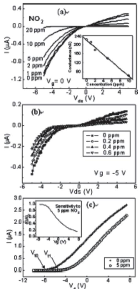
**Figure 10.** (a) ZnO NW I-V curves obtained in different  $NO_2$  concentrations at  $V_g = 0$  V and  $V_g = -5$  V (b) Inset: NW conductance versus  $NO_2$  concentration at  $V_{ds} = -5$  V (c) NW FET I-Vg curves obtained in pure Ar (0 ppm), 5 ppm and 10 ppm  $NO_2$ . Inset: detection sensitivity as a function of gate voltage. (Reproduced<sup>30</sup> with permission from American Institute of Physics, 2005).
