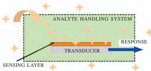
**Figure 1.** Concept of chemical sensor–reaction of the analyte with the sensing layer generate a signal that is converted by the transducer into a measurable response.
