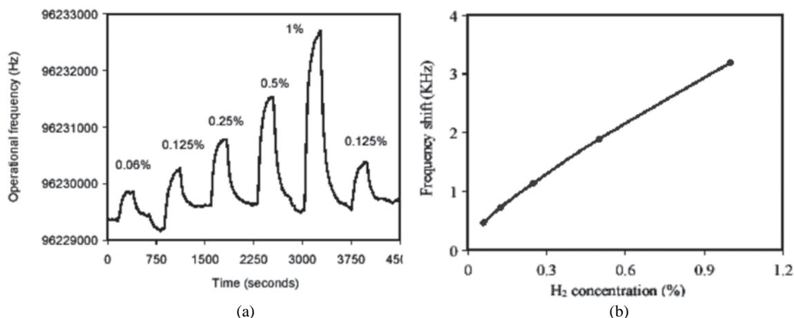
Figure 21. (a) Response of a  $36^\circ\text{YX LiTaO}_3$  SAW-based sensor towards different concentrations of  $\text{H}_2$  gas at  $185^\circ\text{C}$  and (b) Frequency shifts versus  $\text{H}_2$  concentrations (%). (Reprinted<sup>60</sup> with permission from IEEE, 2005).
