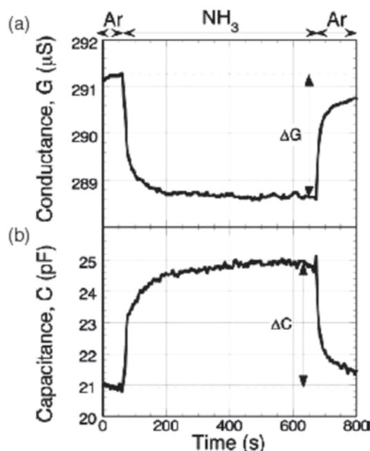
Figure 18. Impedance response of the MWCNT gas sensor to ammonia gas (10 ppm). The sensor was obtained after a 3 h DEP trapping process. The amplitude and frequency of the electrode energising potential were 8 V (peak-to-peak) and 100 kHz, respectively. (a) conductance response, (b) capacitance response. (Reproduced<sup>51</sup> with permission from Institute of Physics, UK, 2003).
