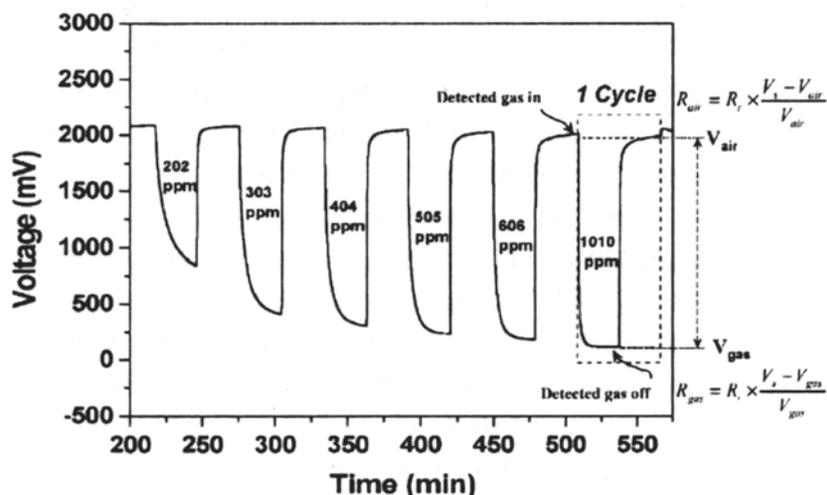
Figure 17. Response curve of hybrid SWCNTs/ $\text{SnO}_2$  sensor to  $\text{NO}_2$  in  $\text{N}_2$  at room temperature. (Reproduced<sup>48</sup> with permission from Elsevier Science, 2004).
