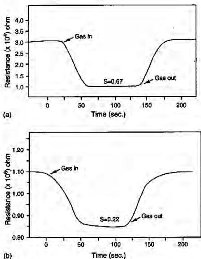
Figure 7. Transient response characteristics of ZnO exposed to 100 ppm  $NH_3$  gas at 300 °C for: (a) nano-ZnO and (b) C-ZnO.
