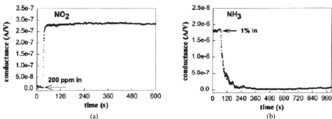
Figure 16. (a) Electrical conductance response of a semiconducting SWNT to 200 ppm  $NO_2$  (b) Electrical conductance response of a semiconducting SWNT to 1 per cent  $NH_3$  vapour. (Reproduced<sup>46</sup> with permission from Science Publishing Group, 2000).
