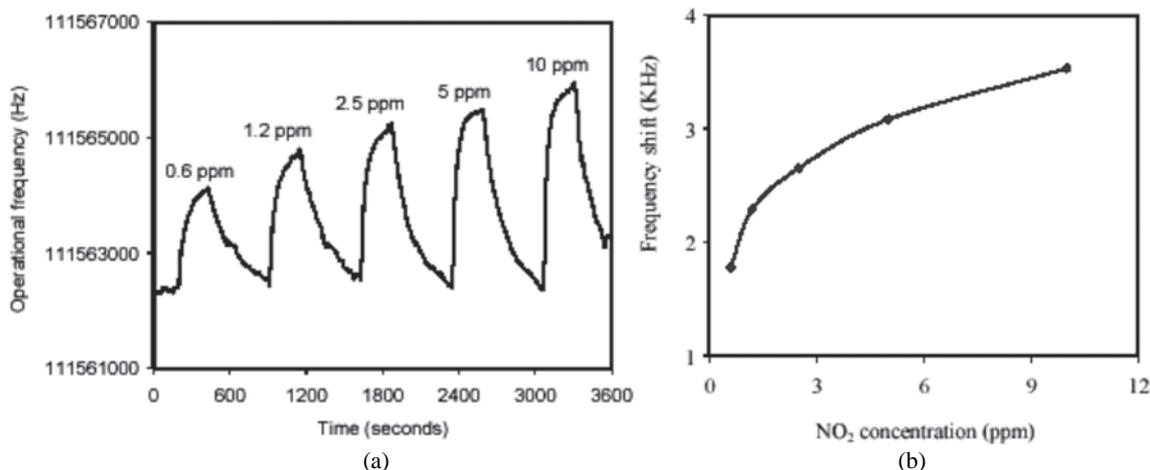
Figure 22. (a) Response of a  $64^\circ$  YX  $\text{LiNbO}_3$  SAW-based sensor towards different concentrations of  $\text{NO}_2$  gas at  $160^\circ\text{C}$ . (b) Frequency shift versus  $\text{NO}_2$  gas concentration (ppm). (Reprinted<sup>60</sup> with permission from IEEE, 2005).
