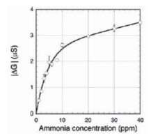
Figure 19. Conductance change of the MWCNTs gas sensor as a function of ammonia. (Reproduced<sup>51</sup> with permission from Institute of Physics, UK, 2003).
