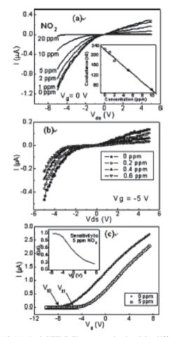
Figure 10.(a) ZnO NW I–V curves obtained in different  $NO_2$ concentrations at Vg = 0 V and Vg = -5 V (b) Inset: NW conductance versus  $NO_2$  concentration at Vds = -5 V (c) NW FET *I–Vg* curves obtained in pure Ar (0 ppm), 5 ppm and 10 ppm  $NO_2$ . Inset: detection sensitivity as a function of gate voltage. (Reproduced<sup>30</sup> with permission from American Institute of Physics, 2005).
