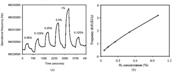
Figure 21.(a) Response of a 36° YX *LiTaO*<sub>3</sub> SAW-based sensor towards different concentrations of  $H_2$  gas at 185 °C and (b) Frequency shifts versus  $H_2$  concentrations (%). (Reprinted<sup>60</sup> with permission from IEEE, 2005).
