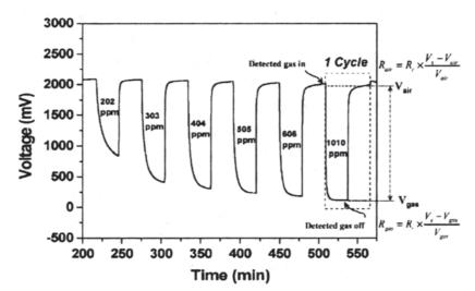
Figure 17. Response curve of hybrid SWCNTs/ $SnO_2$  sensor to  $NO_2$  in  $N_2$  at room temperature. (Reproduced<sup>48</sup> with permission from Elsevier Science, 2004).
