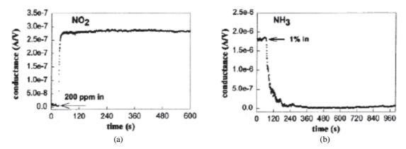
Figure 16. (a) Electrical conductance response of a semiconducting SWNT to 200 ppm NO<sub>2</sub> (b) Electrical conductance response of a semiconducting SWNT to 1 per cent NH<sub>4</sub>, vapour. (Reproduced<sup>46</sup> with permission from Science Publishing Group, 2000).
