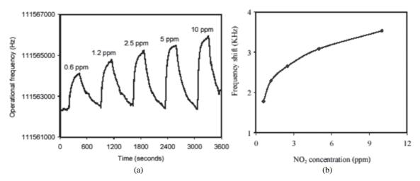
Figure 22. (a) Response of a 64° YX *LiNbO*<sub>3</sub> SAW-based sensor towards different concentrations of *NO*<sub>2</sub> gas at 160 °C. (b) Frequency shift versus *NO*, gas concentration (ppm). (Reprinted<sup>60</sup> with permission from IEEE, 2005).
