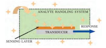
Figure 1. Concept of chemical sensor-reaction of the analyte with the sensing layer generate a signal that is converted by the transducer into a measurable response.
