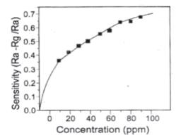
Figure 4. Sensitivity as a function of different concentrations of LPG gas at 200 °C.
