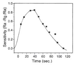
Figure 5. Response of the SnO<sub>2</sub>:Pd thick film to 200 ppm LPG at 200 °C.
