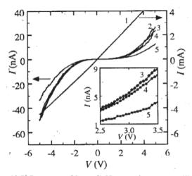
Figure 13.V-I curves of bare GaN nanowires sensor (1) (right hand vertical axis) and a sensor constructed from material of gold nanoparticle-decorated GaN nanowires (curves2-5) (left-hand scale) for in vacuum(2), and atmospheres of Ar(3),  $N_2(4)$ , and methane (5). The inset is an expanded view of the I-V data in the first quadrant ( $\diamond$ : vacuum,  $\diamond$ :  $N_2$ ,  $\blacksquare$ :methane). (Reproduced<sup>36</sup> with permission from American Institute of Physics, 2006).
