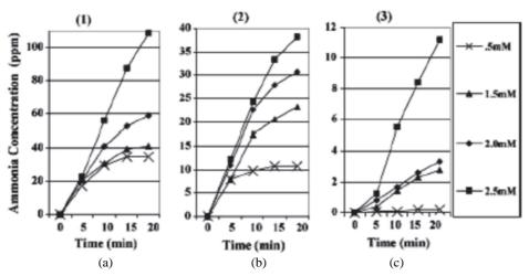
Figure 15. Ammonia concentration versus time when urea solutions reacted with (a) 0.2 ml of urease in PBS buffer, (b) 0.2 ml 30 per cent urease in buffer/70 per cent PVP in ethanol solution, and (c) 0.1 ml of urease/PVP nanofibre material. (Reproduced<sup>44</sup> with permission from Elsevier Science, 2005).
