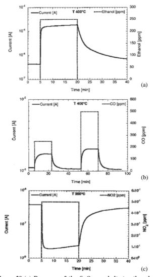
Figure 20.(a) Response of the  $SnO_2$  nanobelts to ethanol at a working temperature of 400 °C and 30 % RH. (b) Response of the  $SnO_2$  nanobelts to *CO* at a working temperature of 400 °C and 30 % RH. (c) Response of the  $SnO_2$  nanobelts to  $NO_2$  at a working temperature of 200 °C and 30 % RH. (Reproduced<sup>58</sup> with permission from American Institute of Physics, 2002).
