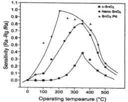
Figure 3. Temperature dependence of the sensitivity of  $SnO_2$ thick films at different operating temperatures.
