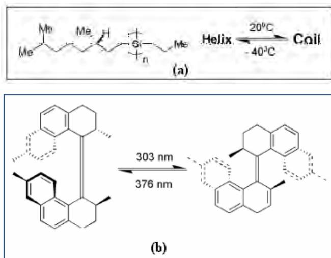
Figure 3. Chemical structures for chiroptical molecular switches: (a) thermo-driven switch of polysilane film<sup>3</sup> and (b) photodriven switch<sup>4</sup>.
