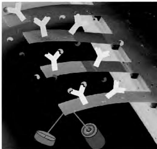
**Figure 15.** Microfabricated cantilevers with surface-immobilised antibodies (gray and yellow symbols) bind only with enantiomers of the correct configuration (red and cyan symbols), detected by the deflection of a laser beam<sup>43</sup>.
