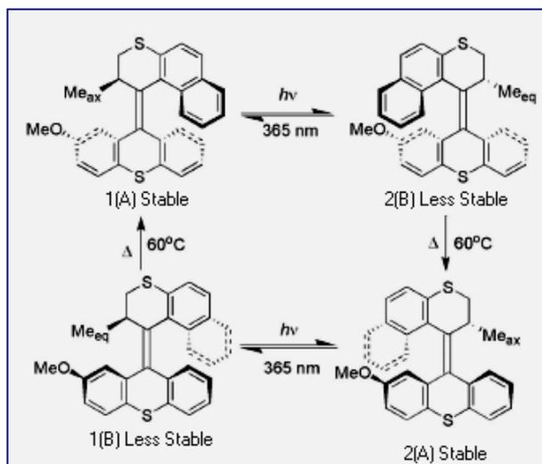
**Figure 6. Different molecular structures and their interconversion for a photo-driven molecular motor system<sup>7</sup>.**
