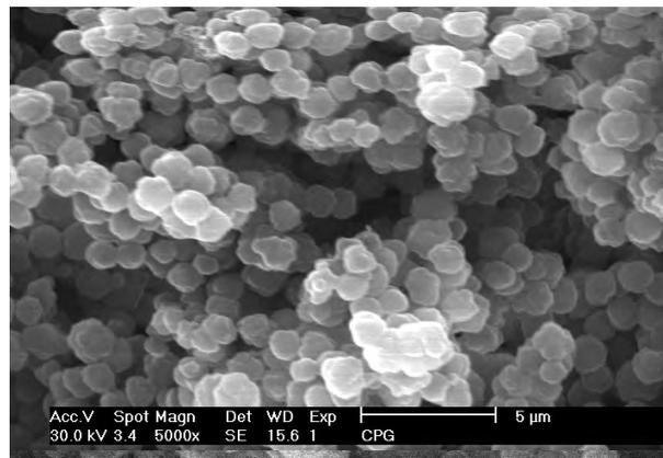
**Figure 16.** SEM micrograph of chiral beads.
