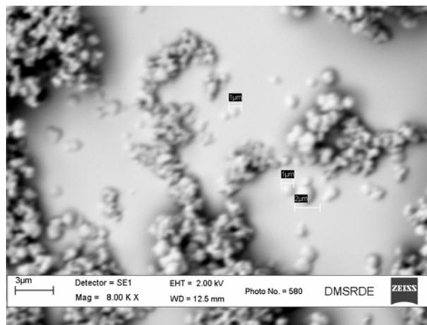
**Figure 17.** SEM micrograph of cross-linked chiral spheres.
