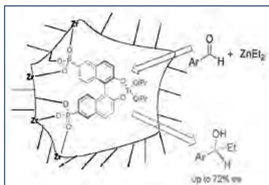
**Figure 11.** Nanoporous zirconium phosphonates containing chiral dihydroxy functionalities used for asymmetric catalysis.
