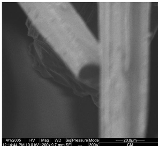
**Figure 18.** SEM micrograph of hollow chiral fibre.
