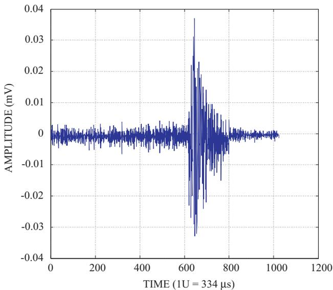
Figure 2. Reference AE signal for crack.
