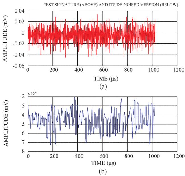
Figure 5. (a) Test-1 data and (b) de-noised data showing signal from hydraulic noise.
