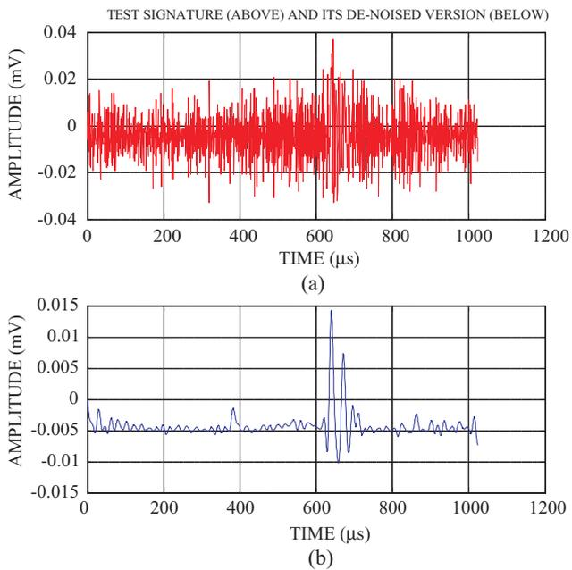
Figure 6. (a) Test-2 data and (b) de-noised data showing signal from a crack.
