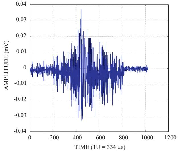
Figure 3. Reference AE signal for rubbing.
