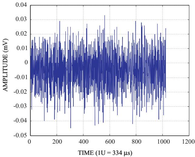
Figure 1. Reference AE signal for hydraulic noise.
