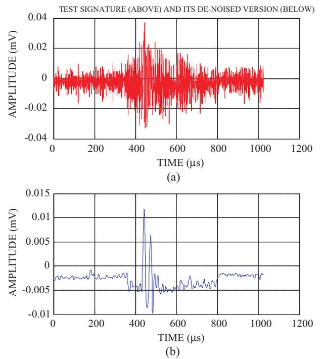
Figure 7. (a) Test-3 data and (b) de-noised data showing signal from rubbing of fasteners.
