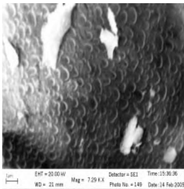
Figure 5. SEM of YAG nanopowder.
