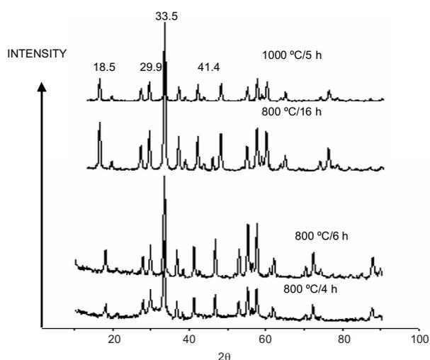
Figure 3. XRD of YAG precursor calcined at different temperatures.
