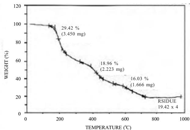
Figure 1. TGA of YAG precursor.
