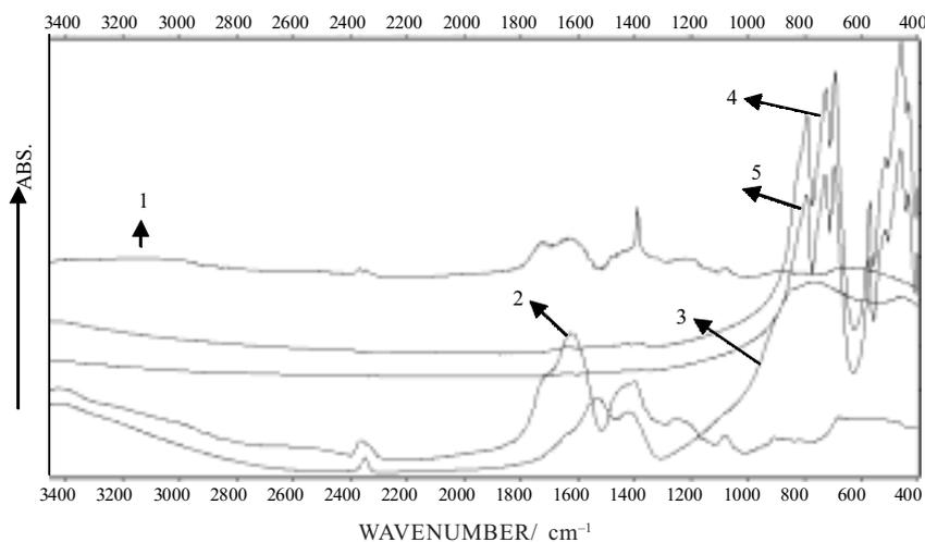
Figure 2. FT-IR of YAG precursor calcined at various temperatures 1-- $110 \text{ }^\circ\text{C}$ , 2-- $140 \text{ }^\circ\text{C}$ , 3-- $650 \text{ }^\circ\text{C}$ , 4-- $800 \text{ }^\circ\text{C}$ , 5-- $1000 \text{ }^\circ\text{C}$ .
