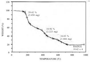
Figure 1. TGA of YAG precursor.
