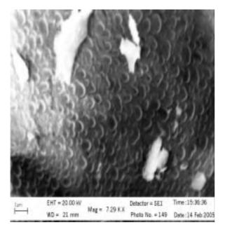
Figure 5. SEM of YAG nanopowder.
