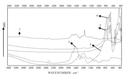
Figure 2. FT-IR of YAG precursor calcined at various temperatures 1--110 °C, 2--140 °C, 3--650 °C, 4--800 °C, 5--1000 °C.
