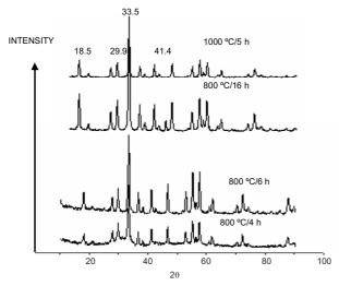
Figure 3. XRD of YAG precursor calcined at different temperatures.
