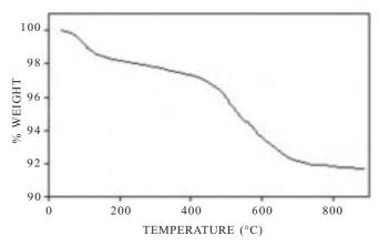
Figure 3. TG curve of washed and dried purified clay (Clay A1).
