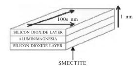
Figure 1. Crystal structure of montmorillonite [(Mg, Al), Si<sub>4</sub>O<sub>10</sub>(OH),].
