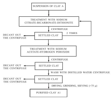
Figure 2. Schematic diagram of purification of Indian clay.
