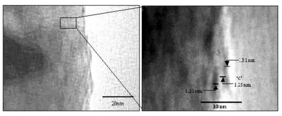
Figure 10. TEM micrograph of purified Clay A1 at high-resolution.
