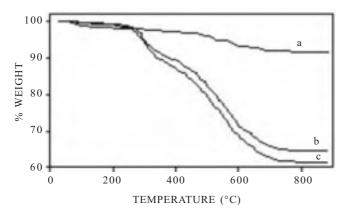
Figure 5. TG curve of: (a) Clay A1, (b) and (c) organicallymodified Clay A1 with salt concentration, i.e., 1.0 CEC of clay and 1.5 CEC of clay, respectively.
