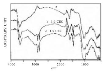
Figure 6. FTIR spectra of: (a) Clay A1, and (b) and (c) organically-modified Clay A1, with salt concentration as shown.
