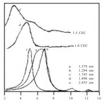
Figure 8. X-ray diffractogram of: (a) clay as such (Clay A),
