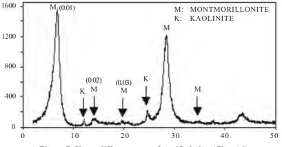
Figure 7. X-ray diffractogram of purified clay (Clay A1).
