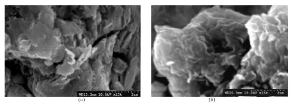
Figure 9. SEM micrograph of: (a) purified clay and (b) organically-modified clay.
