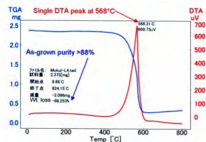
Figure 5. TGA and DTA curves of as-grown CNTs.
