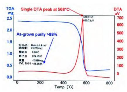
Figure 5. TGA and DTA curves of as-grown CNTs.
