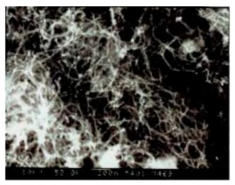
Figure 3. SEM image of as-grown CNTs.
