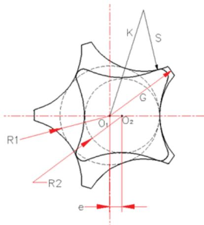
Figure 1. Geometrical parameter of gerotor pump.
