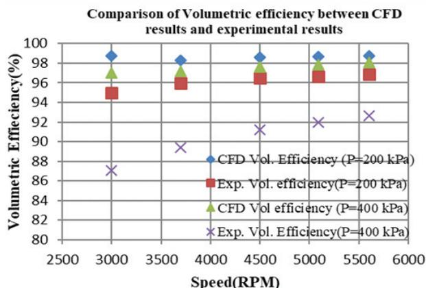
Figure 7. Comparison of volumetric efficiency between simulation result with the experimental result.
