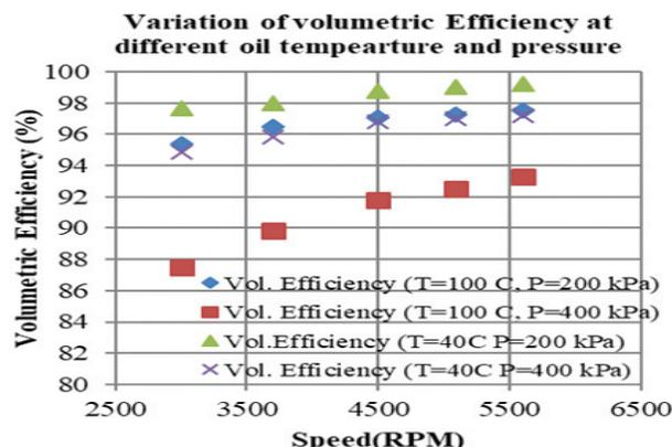
Figure 8. Volumetric efficiency at various operating conditions.
