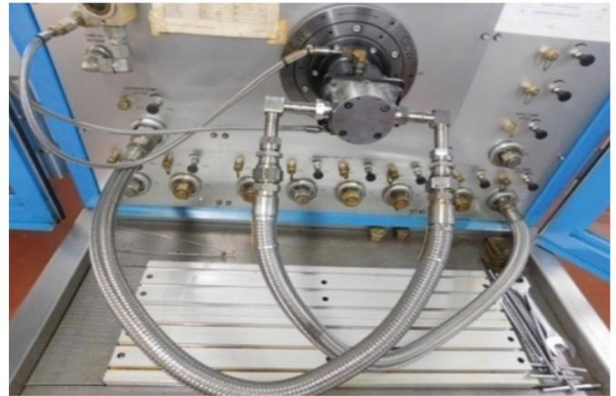
Figure 4. Assembled gerotor pump in the test rig.
