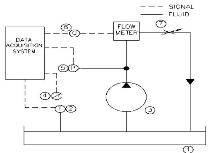
Fig. 5. Layout of the experimental setup.
