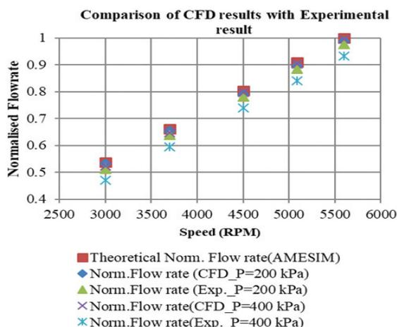
Figure 6. Comparison of Flow rate between simulation result with the experimental result.
