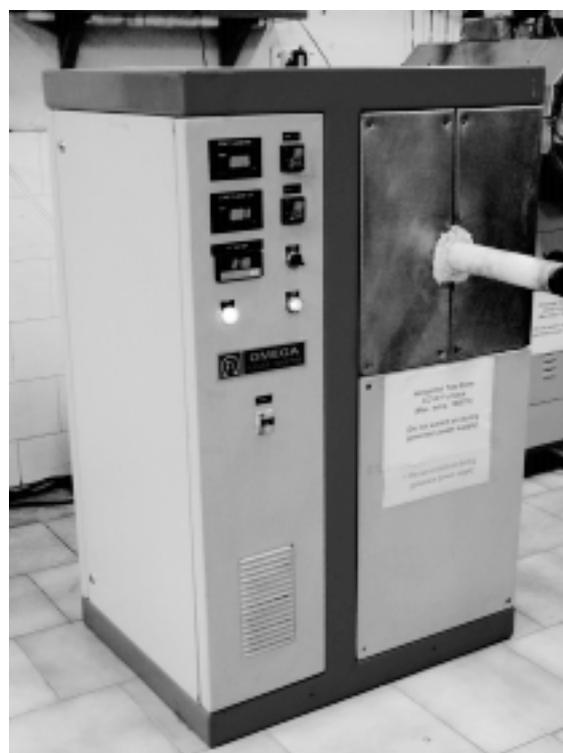
Figure 3(d). High temperature catalytic CCVD furnace (1600 °C).
