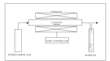
Figure 3(a). Schematic diagram of experimental setup.
