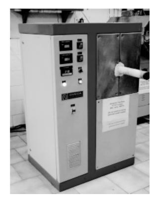
Figure 3(d). High temperature catalytic CCVD furnace (1600 °C).
