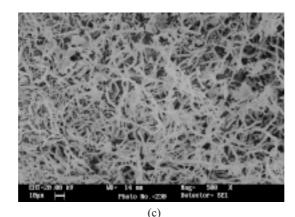
Figure 8. Boron nitride nanotubes synthesised by CCVD method using CNTs as templates.
