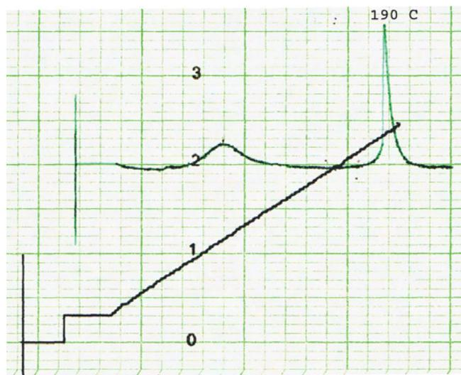
Figure 2. DTA curve of optimised resin CCC formulation.
