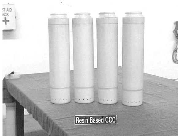
Figure 1. Photograph of resin-based CCC sets before dynamic firing.
