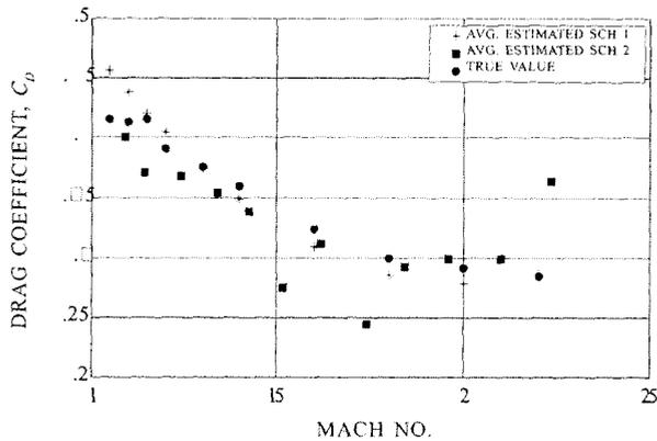
Figure 7. Comparison of average values of estimates through Scheme 1 and Scheme 2 with the true values of drag coefficient.
