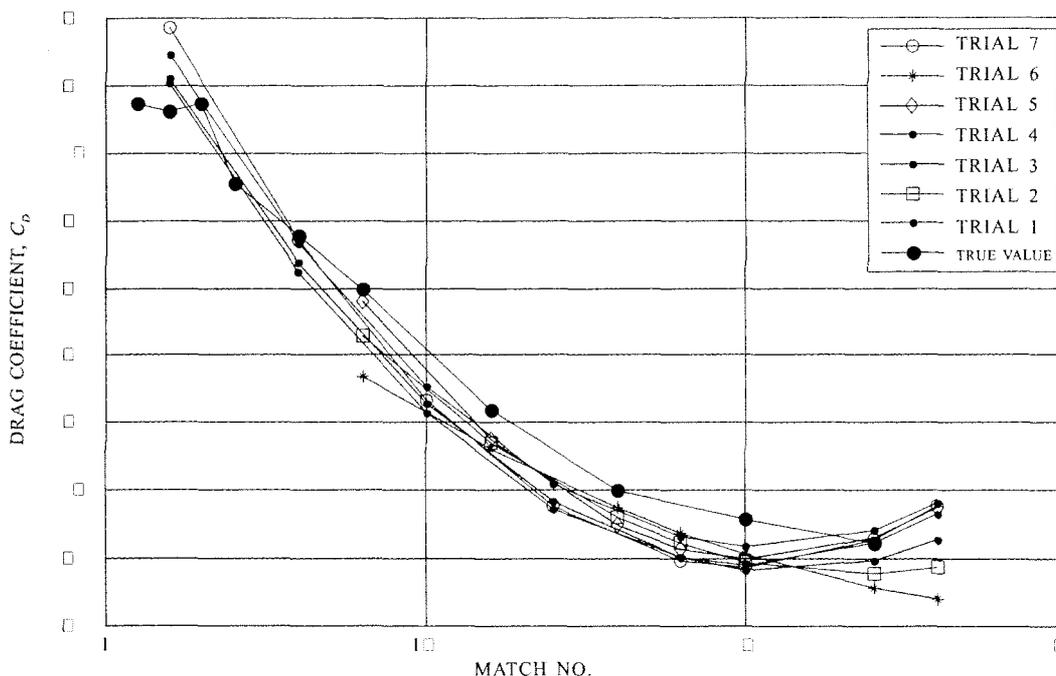
Figure 4. Comparison of estimated values and true values: scheme 1: with initial conditions estimation; Real-flight data.
