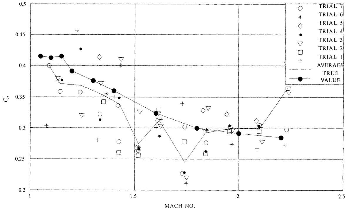
Figure 6. Comparison of estimated and true values of drag coefficient: Scheme 2 (with initial conditions estimation): Real-flight data.
