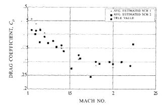
Figure 7. Comparison of average values of estimates through Scheme 1 and Scheme 2 with the true values of drag coefficient.
