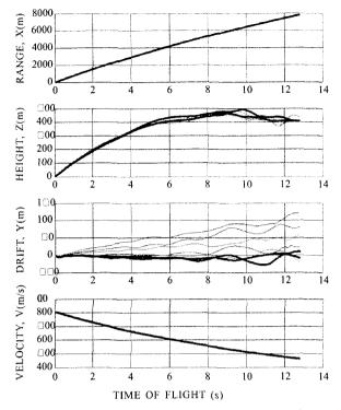
Figure 2. Time histories of real flight trajectory variables of cargo shell.
