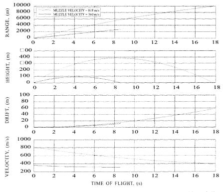
Figure 1. Time histories of trajectory parameters for the chosen artillery shell.
