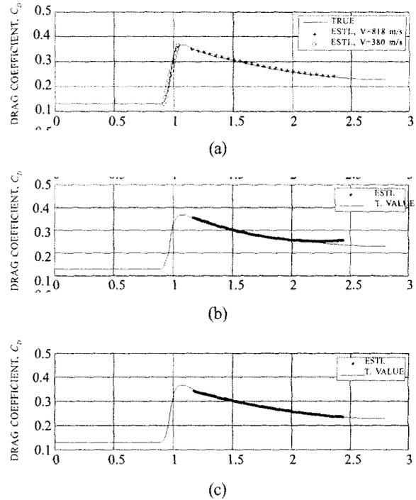
**Figure 3. Comparison of estimated values and true values: Scheme 1: Simulated trajectory data: (a) noise=0 %; (b) noise=5 % (without initial conditions estimation), and (c) noise=5 % (with initial conditions estimation).**
