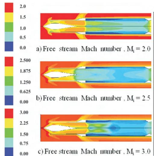
Figure 4. Mach contours for cold air flow.
