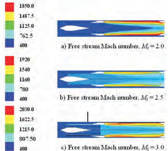
Figure 20. Temperature (K) contours for air/fuel ratio= 30.
