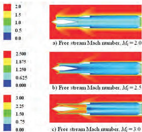
Figure 19. Mach contours for air/fuel ratio= 30.
