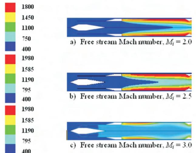
Figure 13. Mach contours for air/fuel ratio = 17.
