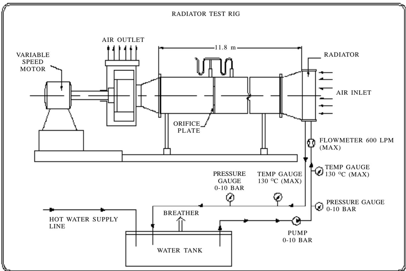
Figure 4. Test setup for radiator performance evaluation.
