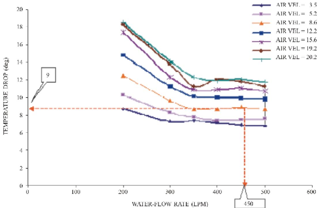
Figure 8. Temperature drop versus water-flow rate (modified radiator-single-pass).
