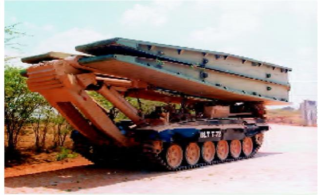
Figure 1. Typical bridge layer tank-T72.
