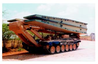
Figure 1. Typical bridge layer tank-T72.
