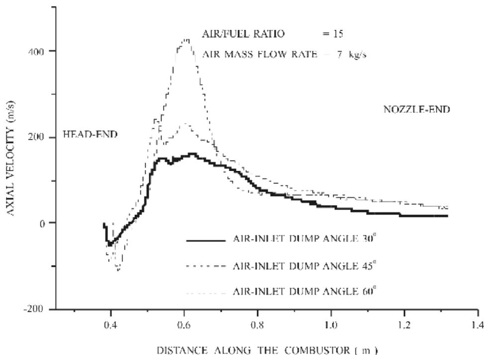
Figure 5. Effect of air-inlet dump angle on centreline value of  $u$  - velocity.
