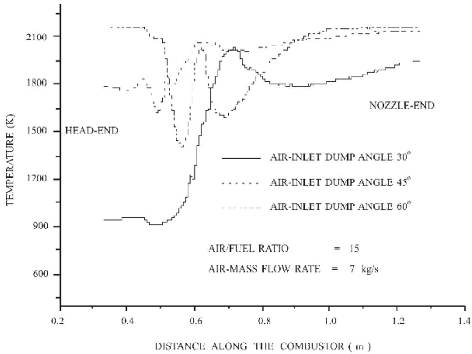
Figure 6. Effect of air-inlet dump angle on centreline variations of temperature.
