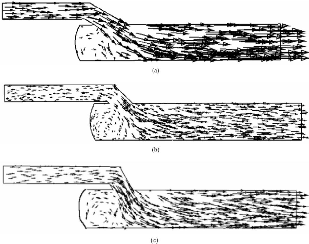
Figure 7. Velocity vectors for different air-inlet dump angles: (a) 30°, (b) 45°, and (c) 60°.
