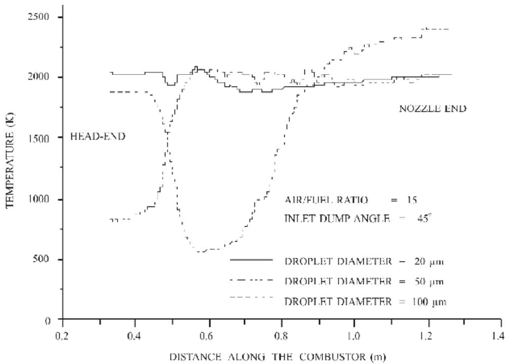
Figure 11. Effect of fuel droplet size on centreline variations of temperature.
