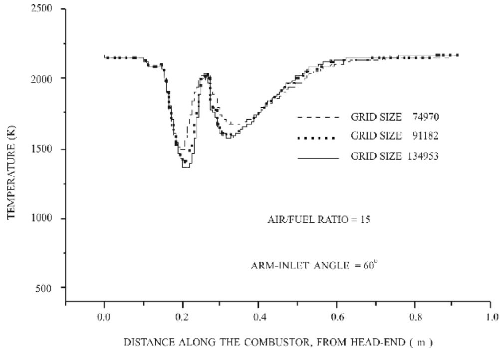
Figure 2. Static temperature variations along the combustor axis.
