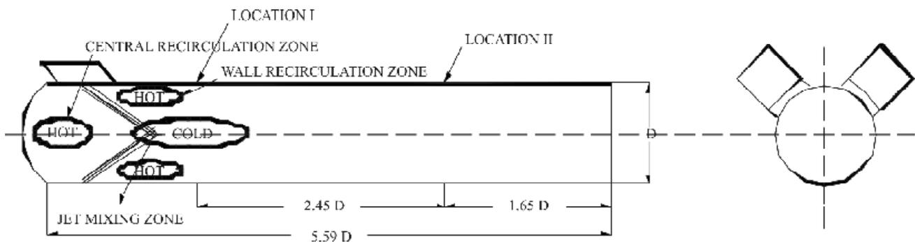
Figure 1. Ramjet dump combustor configuration used for simulation.
