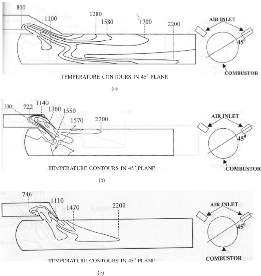
Figure 8. Temperature contours for different air-inlet dump angles: (a) 30°, (b) 45°, and (c) 60°.
