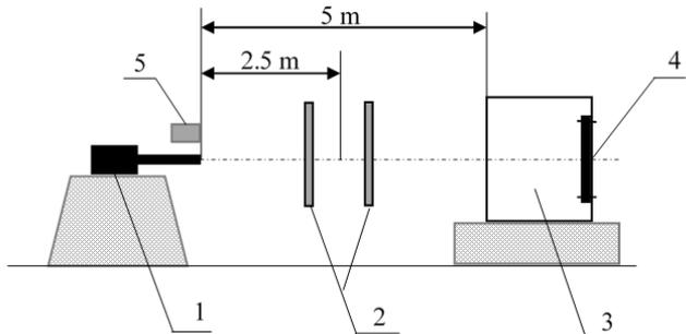
**Figure 3. Scheme of shooting experiment: 1 – ballistic test barrel; 2 – optical gates of ballistic chronograph; 3 – closed steel trap; 4 – flat plate Hardox 450; 5 – ballistic doppler radar.**
