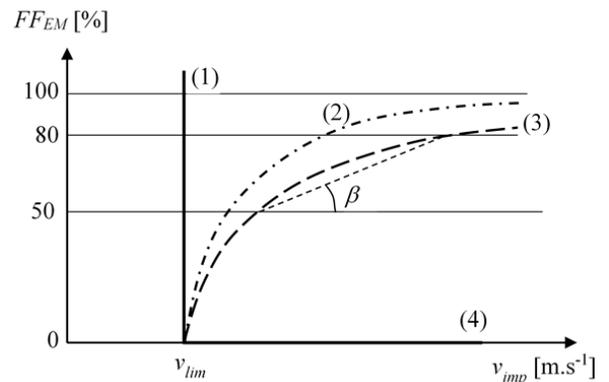
**Figure 1. Typical continuous curve of the dependence of frangibility factor on impact velocity 1 – ideal frangible bullet; 2, 3 – real frangible bullets; 4 – tough bullet.**
