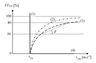
Figure 1. Typical continuous curve of the dependence of frangibility factor on impact velocity 1 – ideal frangible bullet; 2, 3 – real frangible bullets; 4 – tough bullet.
