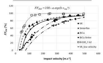
Figure 5. Dependences of frangibility factor on impact velocity for various types of frangible bullet.
