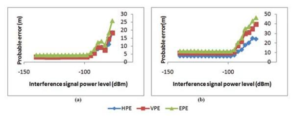
Figure 9. Recorded probable error values for the evaluated GPS receiver at Rio Gallegos for periods of: (a) Best coverage: 0600 (b) Worst coverage: 0300.
